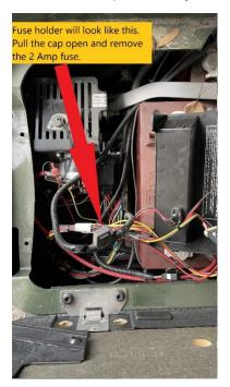
For first-generation RXV ELITE units with lithium batteries, remove the fuse located as indicated below:
